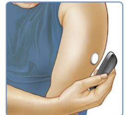
The wireless, rechargeable reader is used to painlessly scan the sensor. This can be done quickly and discreetly, even through clothing. The reader holds up to 90 days of glucose information.
